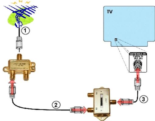
Step 5 Using a fourth coaxial wire (wire #4), plug one end into the other “Out” port on the 2-way splitter. Plug the other end into the “Antenna In (RF)” port on your Converter Box.
