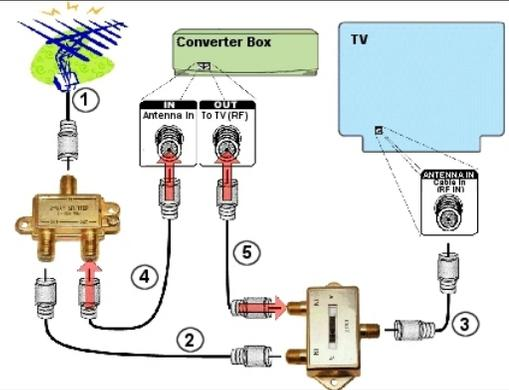
Step 7 Plug the power cords on your Converter Box and TV into a power outlet, and turn on your TV and Converter Box. Set the A/B switch to position “A” and tune your TV to channel 3 (or 4) to watch digital TV. Using the remote control that came with your Converter Box, follow the on-screen set-up guide to scan for available DTV channels, and begin enjoying the benefits of Digital Television! To watch analog TV, set the A/B switch to position “B” and change the channel on your TV set.
